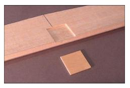
□ Inlay a 1/16" ply control horn pad in the bottom of the elevator. Use the plan as a guide - you will notice that the pad is offset from the center line to better accommodate the control horn. Again, hold off on the actual installation of the horn until later, when it can be aligned perfectly with the installed pushrod. **(R54)**
